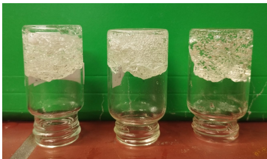
Figure 8. Hydrogels with a rising amount of crosslinking agent DEGDA from left to right (S5, S7.5, S10).
